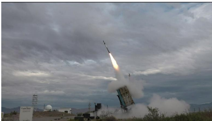
A BQM-177 is launched from the Marine Corps’ Medium Range Intercept Capability system as part of a quad-launch event at White Sands Missile Range, New Mexico.
